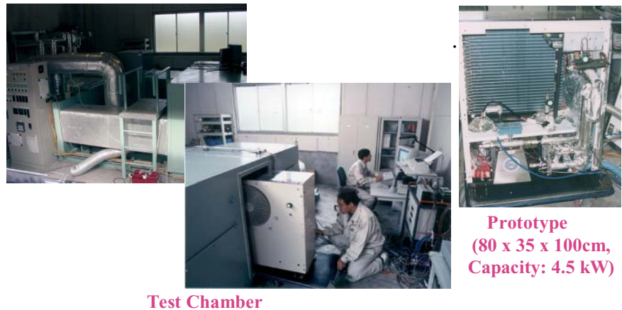
Figure 2: Photograph of the test chamber and the prototype.
